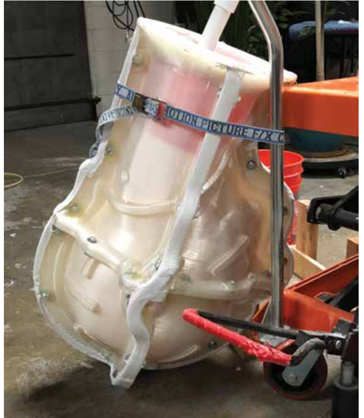
At left, Kazu Hiro's 2017 design for a pour case made using 3D printer software; at right is the actual pour case after being assembled.
